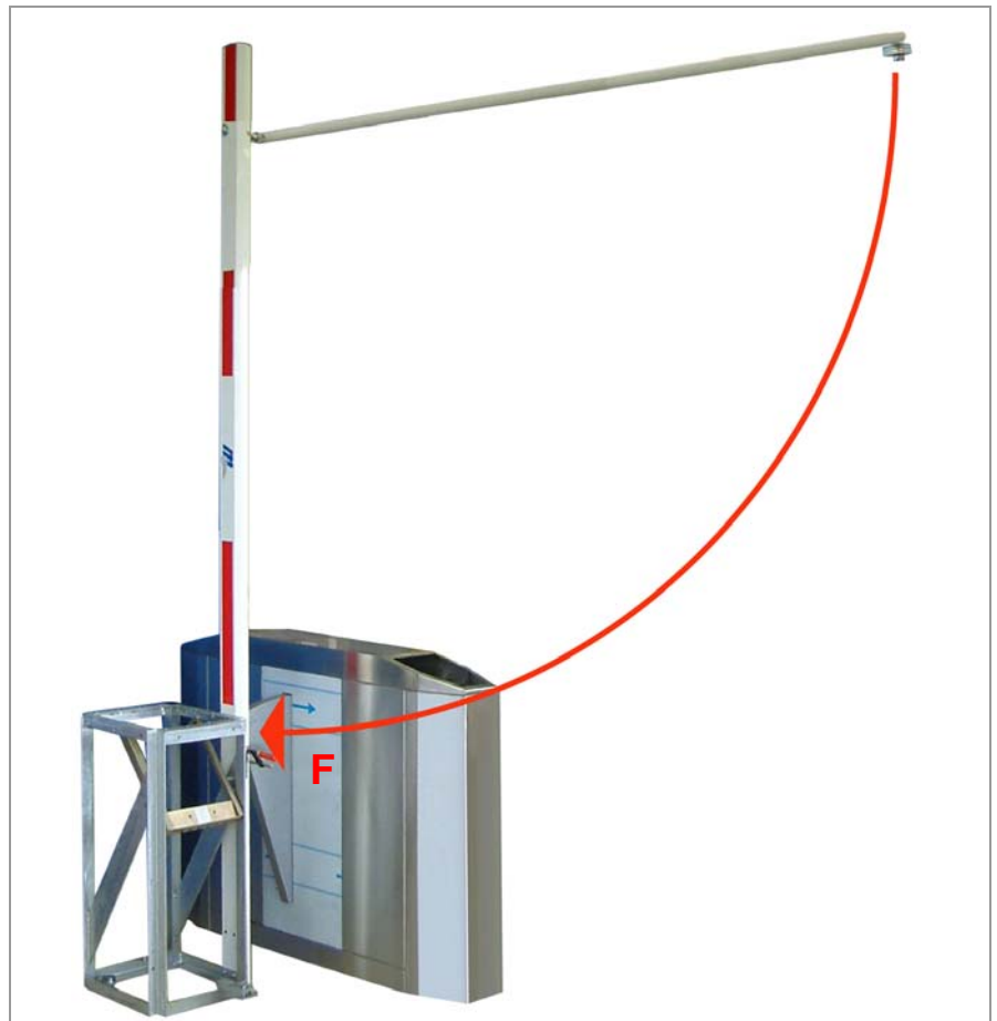
Fig. 3-2 Pendulum impact test; experimental setup with pendulum and weights
